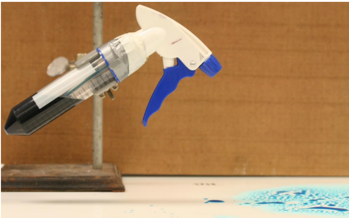
Figure 3.3: Area coverage spray testing set up post spray (side view).
